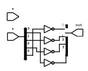
In s? ?:  $\sim$ a, to minimize the amount of logic, the compiler picks  $\sim$ a for the don't-care value ?. This leaves s?  $\sim$ a:  $\sim$ a, which can be simplified to  $\sim$ a. As you can see, the synthesized circuit ignores s and is just  $\sim$ a.
