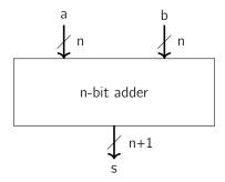
(Remember that n must be fixed in any particular circuit, though – it's not an input.) The way we'll implement this is by using the **standard addition algorithm** we use normally: start adding from the least significant bits and carry a 1 to the next column if necessary. This is better than starting from the truth table, since such a table for a 32-bit adder would give us  $2^{64}$  different rows (which is definitely impossible in practice).
