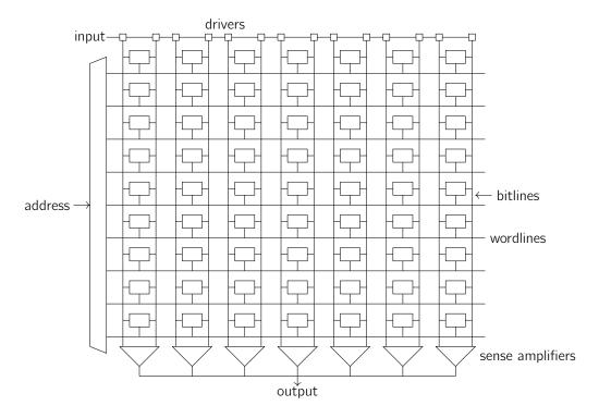
Data comes out of one end of the SRAM. At the output end of each vertical bitline, we have **sense amplifiers**, helping to detect small changes and amplifying them so that outputs are provided more quickly. Finally, data is fed in through inputs from the **drivers** (on the opposite side of the sense amplifiers), and we can write to our SRAM by setting bitlines to appropriate voltages.
