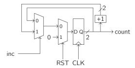
First, we use the reset RST component to initialize our state to 0. Then every time we want to increment our counter, setting inc to 1 allows the circuit to propagate forward that cycle using the wire with the "+1" instead of the wire without it. Here's what this implementation looks like in Minispec:
