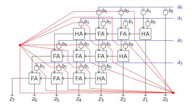
In each pipeline stage, we only have one full adder worth of delay now, meaning that our  $t_{CLK}$  is  $\Theta(1)$  (it's just the amount of time through a single full adder), and we have  $\Theta(N)$  different pipeline stages. So the latency remains  $\Theta(N)$ , but we've **improved our throughput** to  $\Theta(1)$ , which is significantly better. (In words, once we've filled our pipeline, we're able to produce a new valid output once per cycle!)
