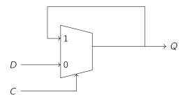
In this circuit, we still have a feedback path that maintains the current state, but we also have a new way to load a value. The multiplexer has an output tied to one of its inputs – if the control signal is 1, then we're using the feedback path where we maintain the old value, so Q holds at its current value. On the other hand, if the control signal C is 0, then we select the input D, and we can propagate the new value.
