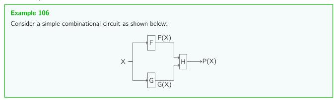
This circuit has three submodules F, G, H, and the latency of this circuit, also known as the propagation delay, is the sum of the times along the slowest path in the circuit. So if we have a latency of  $t_{PD}$ , then the combinational throughput will be  $\frac{1}{t_{PD}}$  (that's how many outputs per second we can produce).
