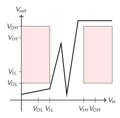
Even though the buffer is just supposed to copy over the input value, it's not good enough to just copy the voltage from  $V_{\rm in}$  to  $V_{\rm out}$  because of noise. And note that our VTC needs to avoid the **forbidden zones** which are shaded above: those are the regions where we feed in a valid input, but we end up with an invalid output.
