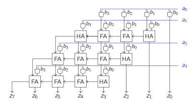
Right now, our latency is of order N for an N-bit adder, because the longest path in the circuit goes across a full ripple-carry adder and also goes down through the various levels, giving us about 2N gates. So using a combinational N-bit multiplier gives us a latency of  $\Theta(N)$  and a throughput of  $\Theta(1/N)$ . (And we can also check that our area is  $\Theta(N^2)$ .)
