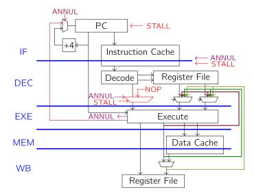
Now, whenever the Execute unit is computing the next PC value, it sometimes finds that we have a jump or a branch that is taken. Then we set the ANNUL control signal to 1, and we supply the mux at the top with the value of nextPC. Furthermore, when we have an ANNUL signal, we have to do **branch annulment**, which replaces instructions in the top two registers (IF-DEC and DEC-EXE) with **NOP**s, and we load the PC register with the correct value of nextPC.
