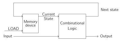
Here, the memory device stores our current state, and the combinational logic device computes two things:
