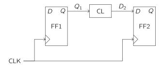
Then we need to make sure that the input  $D_2$  is stable at least  $t_{\text{SETUP}}$  before the next rising edge of the clock, but before that can happen, we need our bit D to propagate through our first flip flop FF1, which then goes through the combinational logic. So we need at least  $t_{\text{PD, FF1}}$  from the first flip flop, plus some time  $t_{\text{PD, CL}}$  to turn a stable Q1 into a stable D2, to all happen early enough. In other words, we need the inequality
