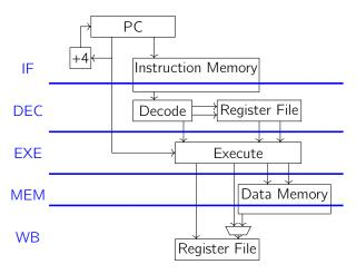
As a clarification, this means that we provide the data value associated with an address **during the next cycle** (if we have a cache hit), rather than in the same cycle. Clocked reads actually **simplify some pipelining issues**, which is why we're using them going forward.
