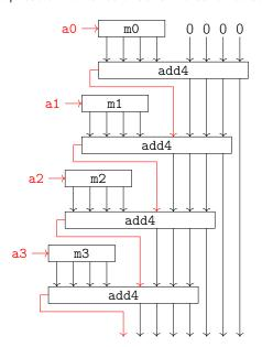
(The left and right inputs into the add4 functions are the two four-digit numbers we add together to keep track of our running total. Notice that after the first addition, our least significant bit is already fixed, and so on.) And now we want to take this further, replacing the add4 functions with actual circuits. We can think about what is actually happening within each box — remember that binary 1-bit multiplication is very easy, because the only time we get a
