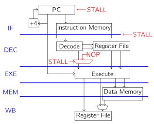
When STALL is 1, the PC doesn't accept a new value, and the IF stage will also keep operating on the same instruction it's been working on (meaning the Decode stage will also still see the same inputs from the previous cycle).
