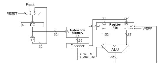
So let's walk through the data flow – once we've fetched and decoded the instruction, we fetch our two source operands, feed them to our ALU along with the **AluFunc**, and feed the information back into the **WD** port (while setting **WE** to 1 so writing is allowed). And this is all the hardware that we need to support register-register ALU operations!
