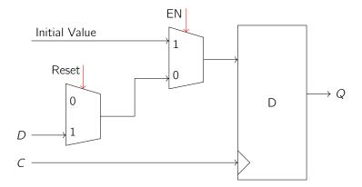
We now have a loadable D flip flop which is capable of remembering its state, loaded with new values, and initalized with certain values. The idea is that whenever Reset is 1, we grab the initial value regardless of the value of EN. But when Reset is 0, we behave like a D flip flop with enable.
