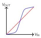
The two endpoints are **stable** here (representing the behavior when we feed in a 0 or a 1), while the middle point is **metastable** – that last point is something we'll return to later in the lecture.
