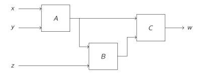
This device is indeed a combinational device as long as A, B, C are combinational devices, because we have digital inputs and outputs, and we can derive a functional description by writing out the function f in terms of the functions of the devices  $f_A$ ,  $f_B$ ,  $f_C$ : it will be
