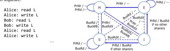
Suppose that Alice and Bob run in two processor cores with private caches, kept coherent with a snoopy, bus-based, write-invalidate MESI protocol (whose state-transition diagram is shown above). Assume write-back, write-allocate caches.
