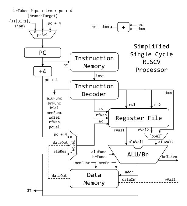
As a reminder, for single-cycle per instruction operation without pipelining, assume that the memory reads (both instruction and data) are combinational, as well as reads from the register file. The instruction decoder decodes the instruction into the following fields:
