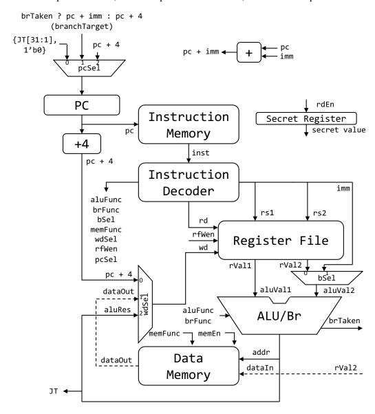
Connect the wires connected to Secret Register to appropriate places on the above diagram. You cannot add additional hardware, other than wires and constants, to this processor. Thus, you need to find a way to use the existing comparator to perform the comparison with <code>0xcafecafe</code>. The multiplexers have been widened for your convenience. If you choose to add additional inputs to multiplexers, indicate so clearly in part (C) if they are to be selected by the multiplexer.
