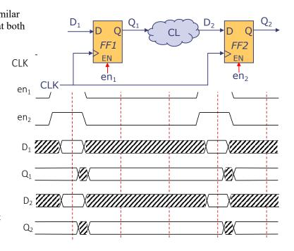
multicycle path: by enabling the registers every third cycle, CL can spend three clock cycles computing each output.
