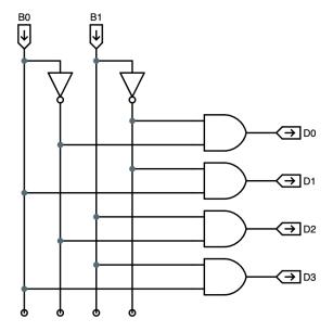
(B) (2 points) Using the block diagram provided to represent your circuit from part (A), add any necessary logic to convert the circuit to a 2-to-4 decoder **with Enable**. If Enable is 0, all output bits should be 0, and if Enable is 1, the outputs should follow the truth table above.
