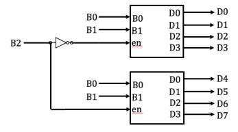
(D) (9 points) Write a parametric recursive function in Minispec that implements a decoder with enable. The two inputs of the function are an n-bit value (b) and a one-bit enable signal (en). The function outputs a 2<sup>n</sup> bit output of all 0s if the enable is 0 and 2<sup>b</sup> if enable is 1. We provided the first line for you to get you started.
