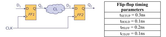
(A)(2 points) If we want t<sub>CLK</sub>=1ns, what is the maximum propagation delay of the combinational logic CL? What is the minimum contamination delay of CL for the circuit to work properly?
