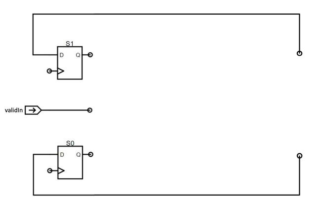
(E) (2 points) Suppose that we implement the flip-flop with enable using a normal D flip-flop without an enable and a mux, as shown below. Will any mux implementation work correctly? If so, explain why. If not, give an example of how an inappropriate mux implementation could cause metastability.
