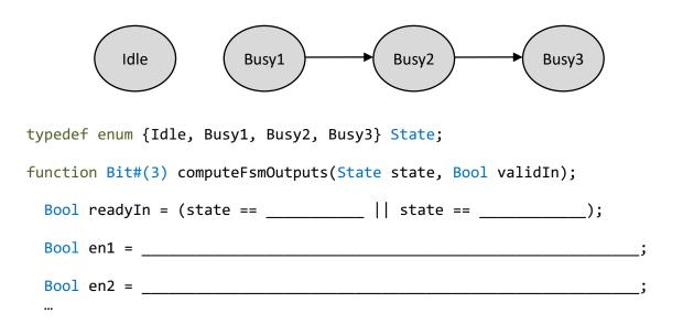
(D) (5 points) Assume that states are encoded using 2-bit values as shown to the right. Use your FSM from part C to fill in the truth table below. Then implement the combinational circuit that computes the next state (*nextS1, nextS0*) given the current state (*S1,S0*) and the *validIn* input. Use the **validIn** input and **S1** and **S0** registers provided below. You can use NOT, AND, OR, and XOR gates. For full credit, your circuit should not use more than eight gates.
