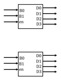
(D) (9 points) Write a parametric recursive function in Minispec that implements a decoder with enable. The two inputs of the function are an n-bit value (b) and a one-bit enable signal (en). The function outputs a 2<sup>n</sup> bit output of all 0s if the enable is 0 and 2<sup>b</sup> if enable is 1. We provided the first line for you to get you started.
