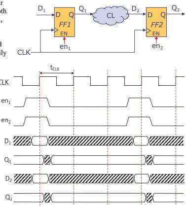
(B) (4 points) If we want  $t_{CLK}$ =1ns, what is the maximum propagation delay of the combinational logic CL in the above 3-cycle path? What is the minimum  $t_{CD}$  for the circuit to work properly?
