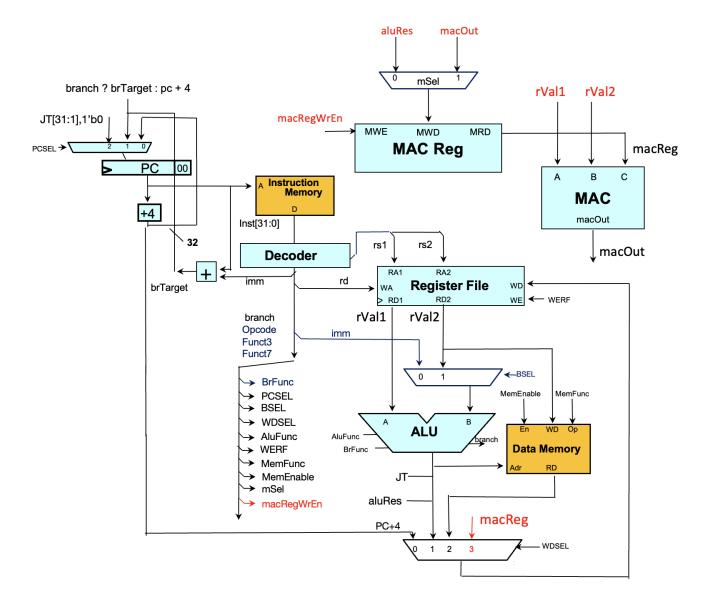
(D) (4 points) What does the decoder need to output for the following fields if given the instruction macw x0, 0x100 and macr x10? Add any additional signals you may have added in part C. Mark any Don't Care values with a?
