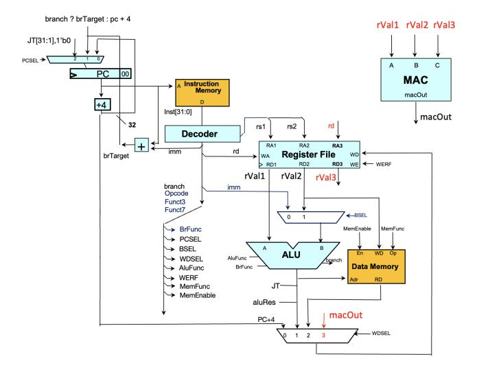
(B) (4 points) What does the decoder need to output for the following fields if given the instruction mac1 x2, x5, x10? Add any additional signals you may have added in part A. Mark any Don't Care values with a?
