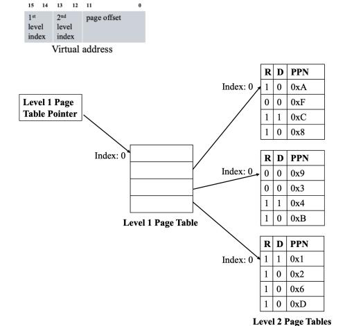
Translate the following virtual addresses to physical addresses using this two-level hierarchical page table. If a virtual address does not map to a physical address according to the diagram above, then write PAGE FAULT.
