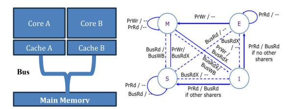
We examine a new sequence of accesses on addresses X and Y. Fill in the following table showing the bus transactions that result from each access, and the cache contents, along with the state of each line. **Each cache can hold only one line**. Clearly indicate the line in the cache and its state (e.g., "X: I", "Y: S", etc.). If there are multiple bus transactions, list them in order.
