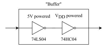
(A) (2 points) If Ben chooses a supply voltage of  $V_{DD} = 5V$  for the CMOS chip (74HC04), the specifications for the CMOS chip become:  $V_{OL} = 0.15 \text{ V}$ ,  $V_{IL} = 1.5 \text{ V}$ ,  $V_{IH} = 3.5 \text{ V}$ ,  $V_{OH} = 4.85 \text{ V}$ . With this supply voltage, Ben's circuit does not correctly function as a buffer. Explain why the buffer does not work with this supply voltage. Provide a concrete example in your explanation.
