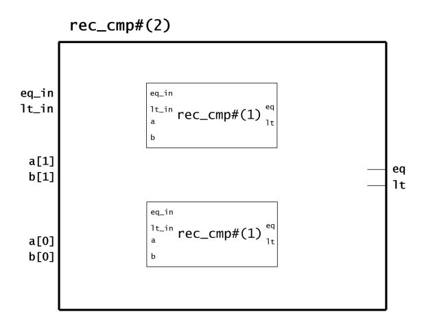
Consider the same circuit for a general parameter n. How does the propagation delay of the circuit grow with n? Provide an explanation for why this is the propagation delay for this implementation.
