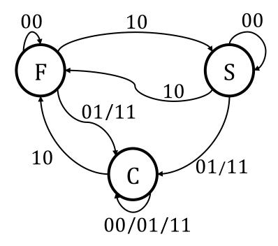
If the baby is in the Slept state (S) and it cries but doesn't smell, what state does this FSM go to?
